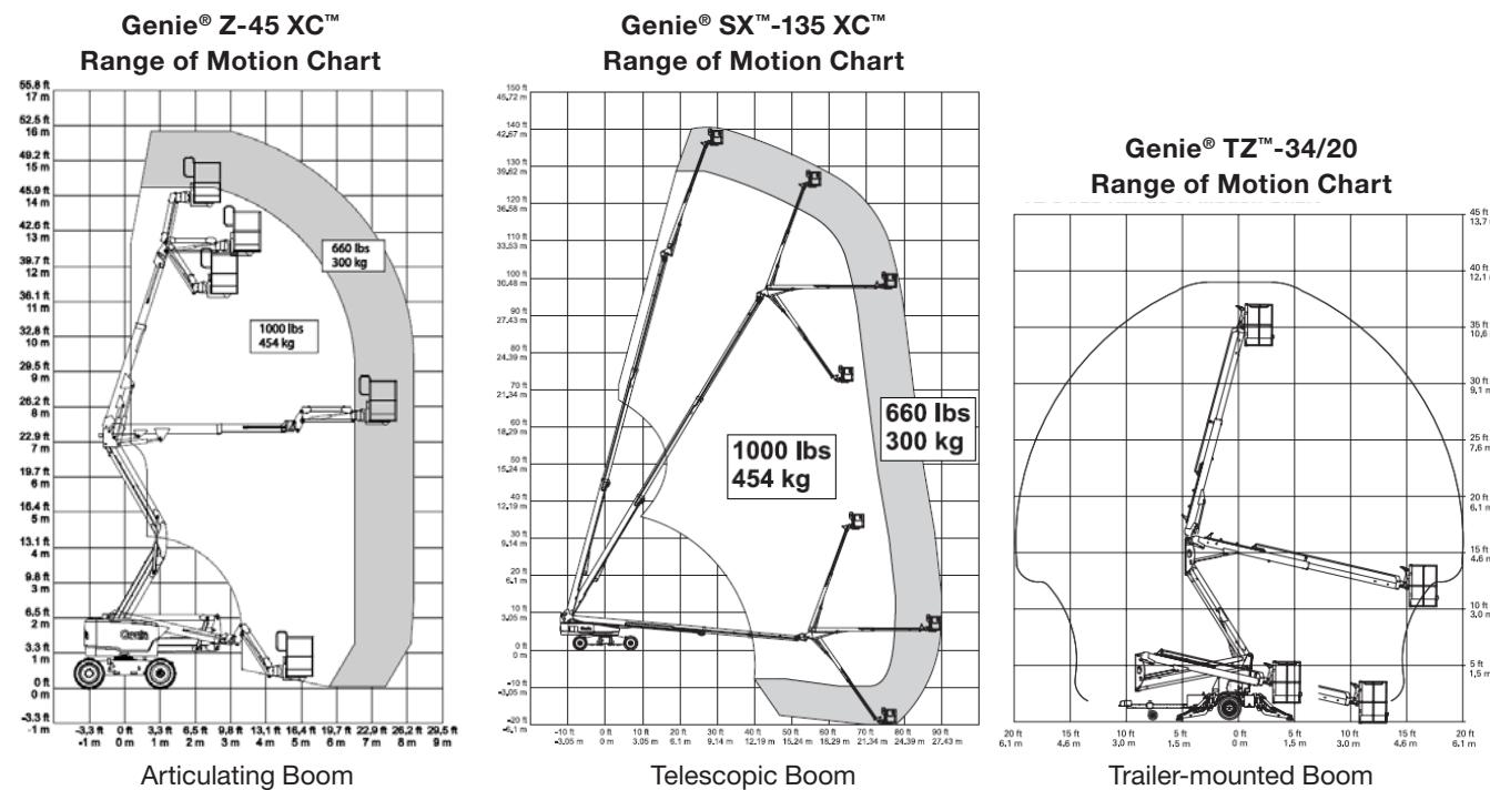
Model numbers often reflect the maximum reach capabilities of the machine's platform or deck [e.g., Genie® SX™-135 XC™ designates a 135 ft (41.15 m) stick boom].
